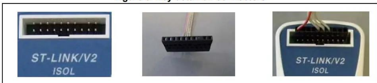
Figure 6. Key detail on connectors
