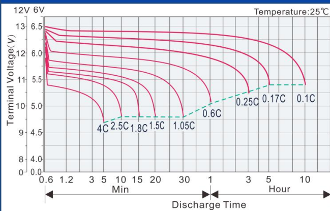
Discharge characteristic curve (25°C/77°F)
