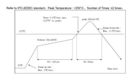
Figure 6 Recommend reflow soldering temperature curves
