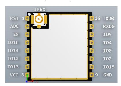
Figure 2 ESP-07S pinout
