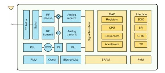
Figure 1 ESP8266EX Functional Block Diagram
