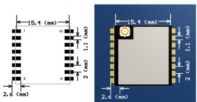
**Figure 5 Module PCB Footprint**
